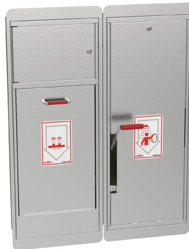
a stainless steel handle extending out of the cabinet. The cabinet will have an integral access panel to allow access to the emergency-mixing valve. The eye/face/wash portion shall be housed in an 18-gauge, Type 304 stainless steel cabinet to conceal and protect the fixture.
